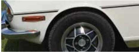
*At the front, both stripes are broken, curved at a radius of 30mm from wing edge*
