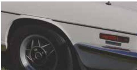
*Bottom of thick stripe is 16mm above the rear badge at highest point. Cut is in the thick stripe only over the wheel arch at a radius of 30mm from the wheel arch. The thin top line continues straight across the top of the wheel arch*
